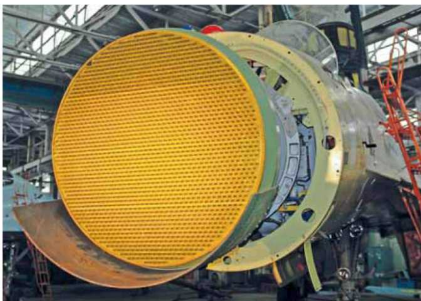
Fig. 4. Irbis fire control radar
